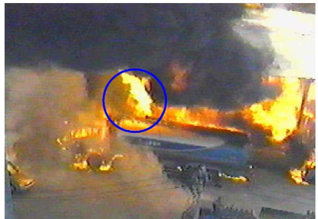
Fig. 7. Flame surrounding butane tank lorry and small flame by purged butane through safety valve.
