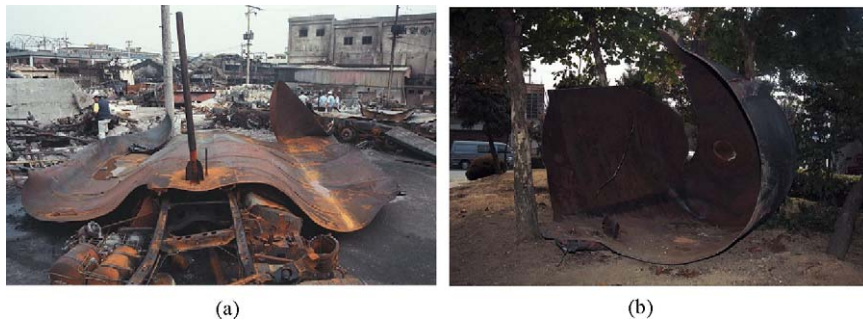
Fig. 9. Butane tank lorry after explosion: (a) body and (b) front part of tank.
